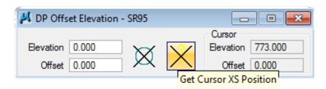
**Move** your cursor around in the view. The Elevation and Offset readings are displayed in the tool.
